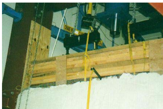
Figure 7: View of top plate, ram and measuring tape. (Photograph P. Florence)
