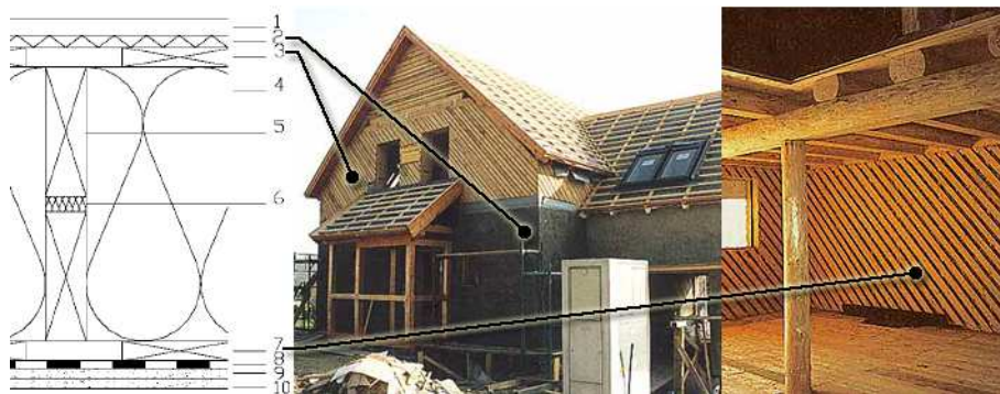
Figure 4.9: One of the first prefabricated straw bale houses in Breitenfurt in Austria. Wall section on the left : 1 — light, silicate based exterior plaster, 2 — cement based wood wool panel (heraklith), 3 — diagonally clad timber, 4-6 — straw bales between double timber studs, 7 — diagonally clad timber, 8 — vapour barrier, plastic sheet, 9 — gypsum plasterboard, 10 — interior plaster. Image of exterior of the house under construction is in the middle and interior, prior to sheeting with "vapour" barrier, is on the right . Section is from Wimmer et al. (2001) and images from www.baubilogie.at .
