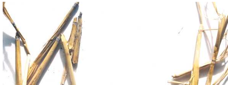
Figure 4.18: February 17th 2006 (12 weeks after the damage). Both samples smelled strongly of mold. On the left is a sample taken approximately 50mm from the exterior plaster. The straw has large dark spots on the stems. The nodes are completely black. On the right is sample taken approximately 100mm from the exterior plaster. About half of the nodes are darkened. The stems have a healthy colour.
