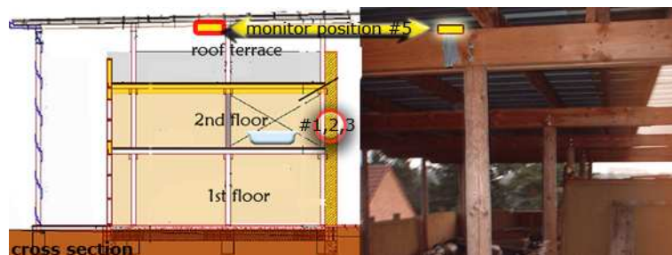
Figure 6.5: Straw bale house in Blanden, Belgium. The external monitor #5 was fixed to the top of the roof joist just under the metal roof (see yellow arrow ) far from the internal monitors #1,2,3 (see red circle ).
