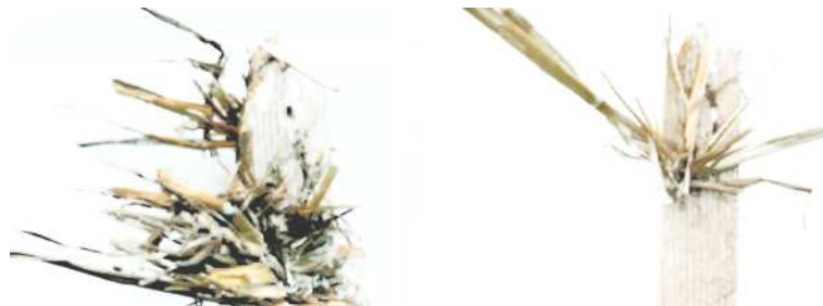
Figure 4.20: September 20th, 2006 (10 months after the damage). Both samples smelled of mold. On the left is a sample taken approximately 30mm from the exterior plaster. The black straw shows signs of decomposition. The nodes are completely black. On the right is a sample taken from mid-wall-depth. After 10 months in an environment with a high humidity level (above 70%) the straw is not visibly damaged.
