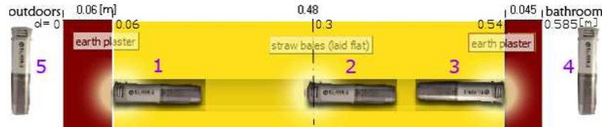
Figure 4.22: Relative humidity and temperature data inside the bathroom's external wall in the family house in Blanden were monitored by three dataloggers. #1 was placed in the straw just under the exterior earth plaster, #2 in the middle of the bale and #3 in the straw just under the interior earth plaster. 2 other dataloggers were placed externally. Monitor #4 in the interior of the bathroom and monitor #5 outside.
