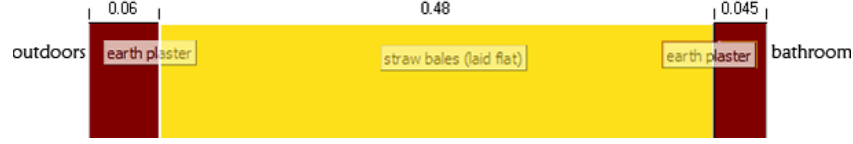
Figure 5.2: Section through the external bathroom straw bale wall in Blanden (see case study II., Section 4.2.2). The straw bales are laid flat \Rightarrow the heat and water vapour flow are parallel to the straw fibre. A commercially produced earth plaster (CLAYTEC, Lehm Unterputz) was mixed with water and sprayed in three layers onto both sides of the straw bales.
