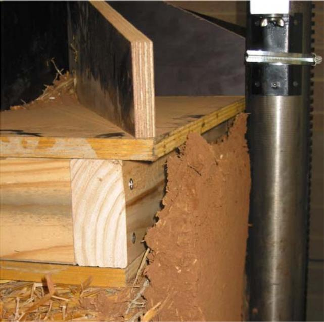
Figure 10 ‘Sinking-in’ of the top-loading frame (Note how render has behaved)
