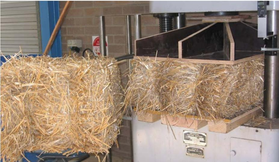
Figure 5. Compressed state of the straw bale
