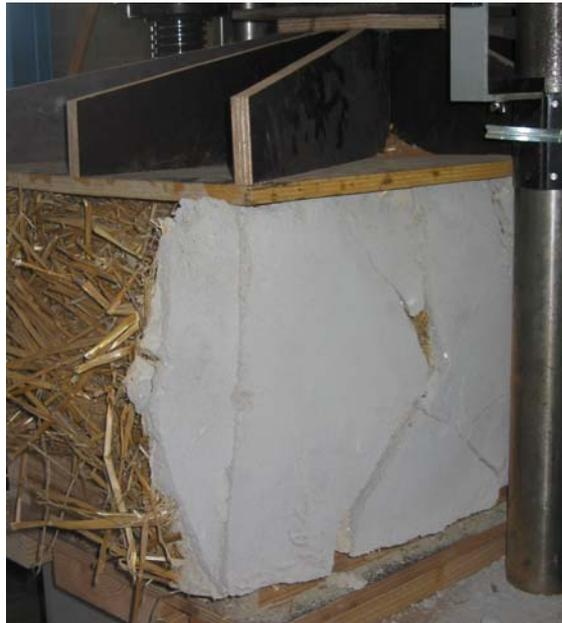
Figure 14 Loading of both bale and cement render directly (note cracking pattern)
