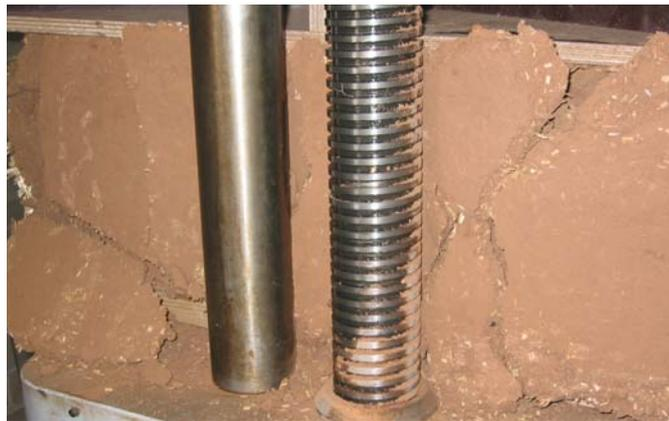
Figure 12 Cracking in earth render at the end of the test
