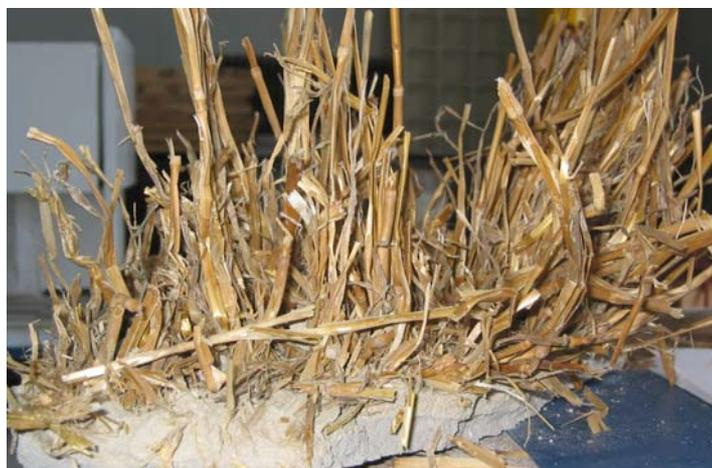
Figure 16 Bonding between straw and cement render
