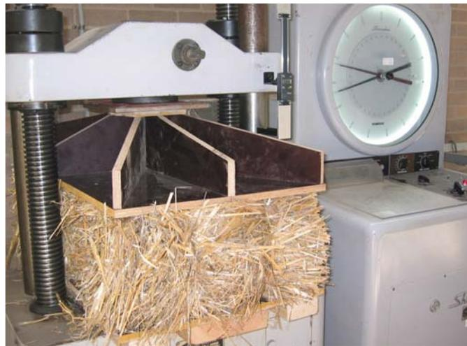
Figure 2 Test set-ups for unrendered strawbale test
