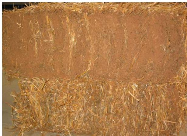
Figure 13 Difference in adhesion on two sides of the bale
