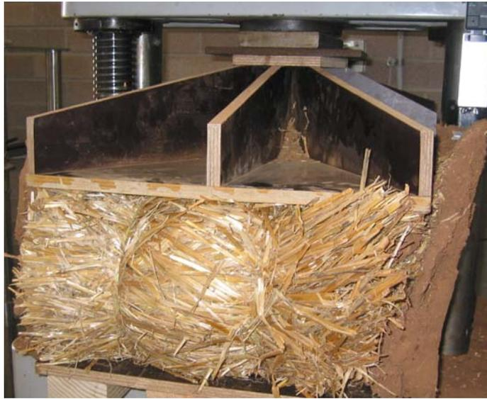
Figure 11 Final compressed state of earth rendered strawbale
