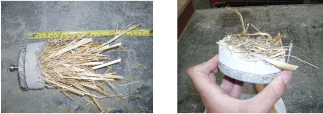
Fig. 6: Example of pull off disc from flat (left) and on-edge (right) wheat bales.
