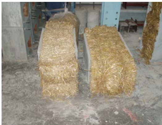
Fig. 10. Straw bales plastered on-edge (left) and flat (right).
