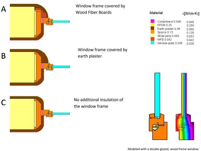
Aodeled with a double glazed, wood frame window: Uframe = 1.38W/m^2K\*
