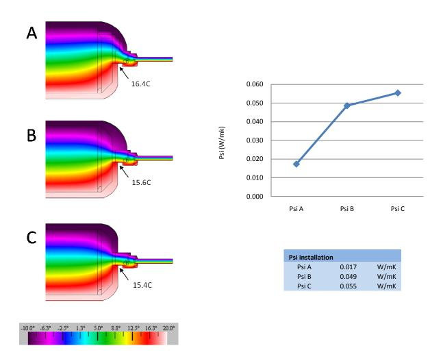
The results show that the use of wood fiber boards (case A) can improve the installation psi value more than three times, when compared to the window frame exposed directly to the external environment (case C). Conversely, covering the window frame with earth plaster (case B) does not make a big difference from the direct exposure of the frame to the exterior.
