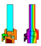
Modeled with Optiwin Zwoa2Holtz PHI certified window. wooden frame, cork insulated, triple glazed, Uframe (sill) = 1.05W/m^2K\*
