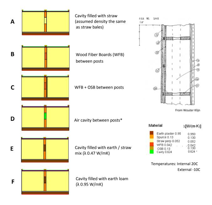
\* The air cavity thermal resistance determined as per ISO EN 6946
