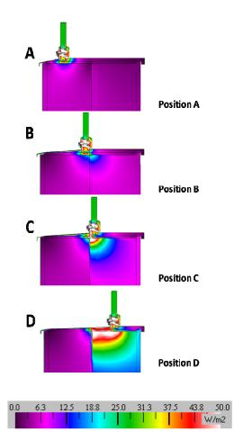
The heat flux is highest at the original position of the window (case D). The heat flows through the layer with the higher thermal conductivity (masonry) directly to the external environment and the insulation (straw) is doing a little to prevent this. The non optimized placement of the window leads to significant thermal bridging and associated thermal losses.
