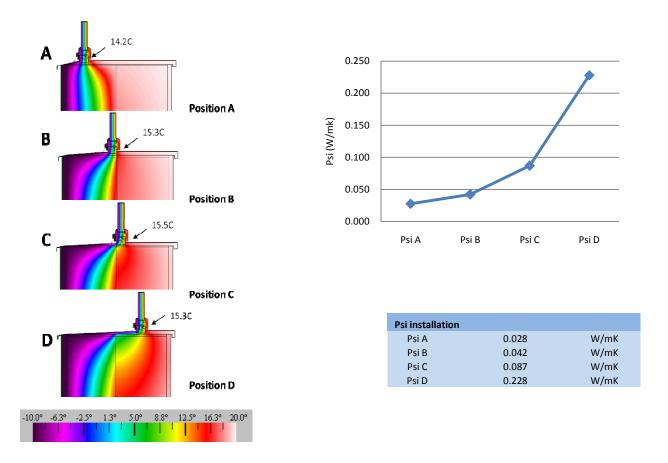
The simulation shows that the difference in Psi value between cases A and D is more than eighth fold. This would lead to a significant increase of the overall U-value of the building envelope.
