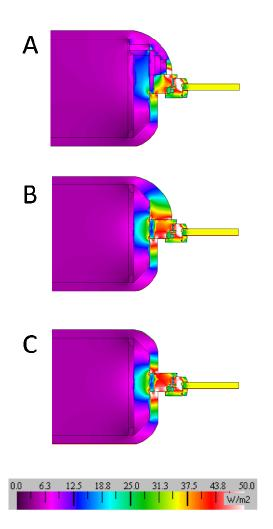
The wood fiber boards reduce the heat flow from the internal to the external environment. The earth plaster (case B) is not able to fulfill the same role. The exposure directly to the exterior (case C) leads to even higher heat flow.
